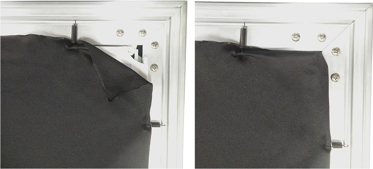
3. Secure the remainder of the black backing. The black backing should now be secured at the corners, but will be loose along the edges. At the center and several other mounting points along each edge, release the springs from the screen tension rods and lay the black backing over the rod, then reattach the springs. This will effectively tuck the black backing between the tension rod and each spring so that it will be secured in place. Your black backing is now properly installed.
