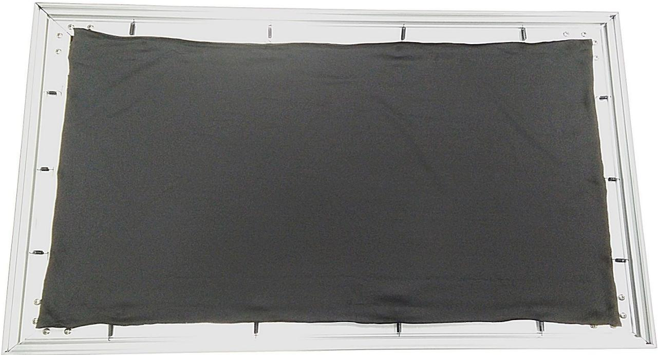
2. Secure the black backing at each corner. Release the two springs closest to each corner from the tension rods. Lay the black backing over the rod and hook the springs back over the tension rod and the black backing. Tuck the very corner of the material behind the tension rods to hold it firmly in place.
