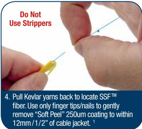
4. Pull Kevlar yarns back to locate SSF™ fiber. Use only finger tips/nails to gently remove "Soft Peel" 250um coating to within 12mm / 1/2" of cable jacket.<sup>1</sup>
