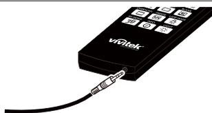
**Wired Remote Jack** Connect to WIRED REMOTE terminal on the projector
