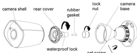
Loosen (but do not remove) the set screw on the side of the camera. Remove the camera assembly from the base. Remove the rear cover. Open the waterproof lock and remove the lock nut and rubber gasket.
