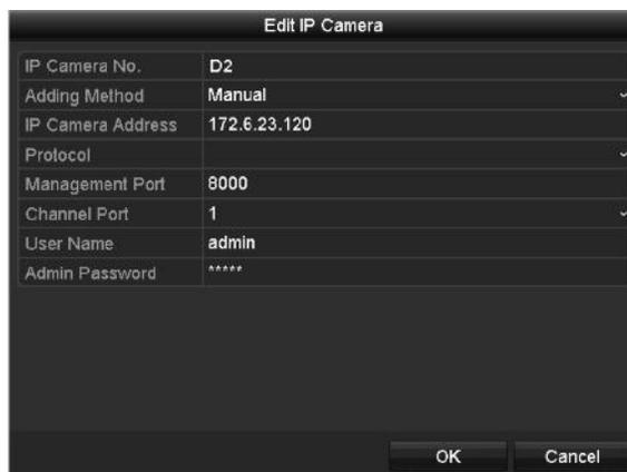
Figure 2. 24 Edit IP Camera Interface - Manual
