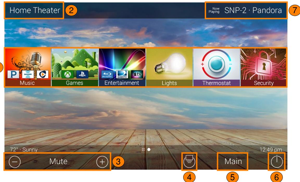
5. **Main:** Select to return to the Main Menu regardless of what page the device is currently on. This can be changed to display the Scenes Menu, speak with the custom integrator to program the TDC-9100 in this way.
