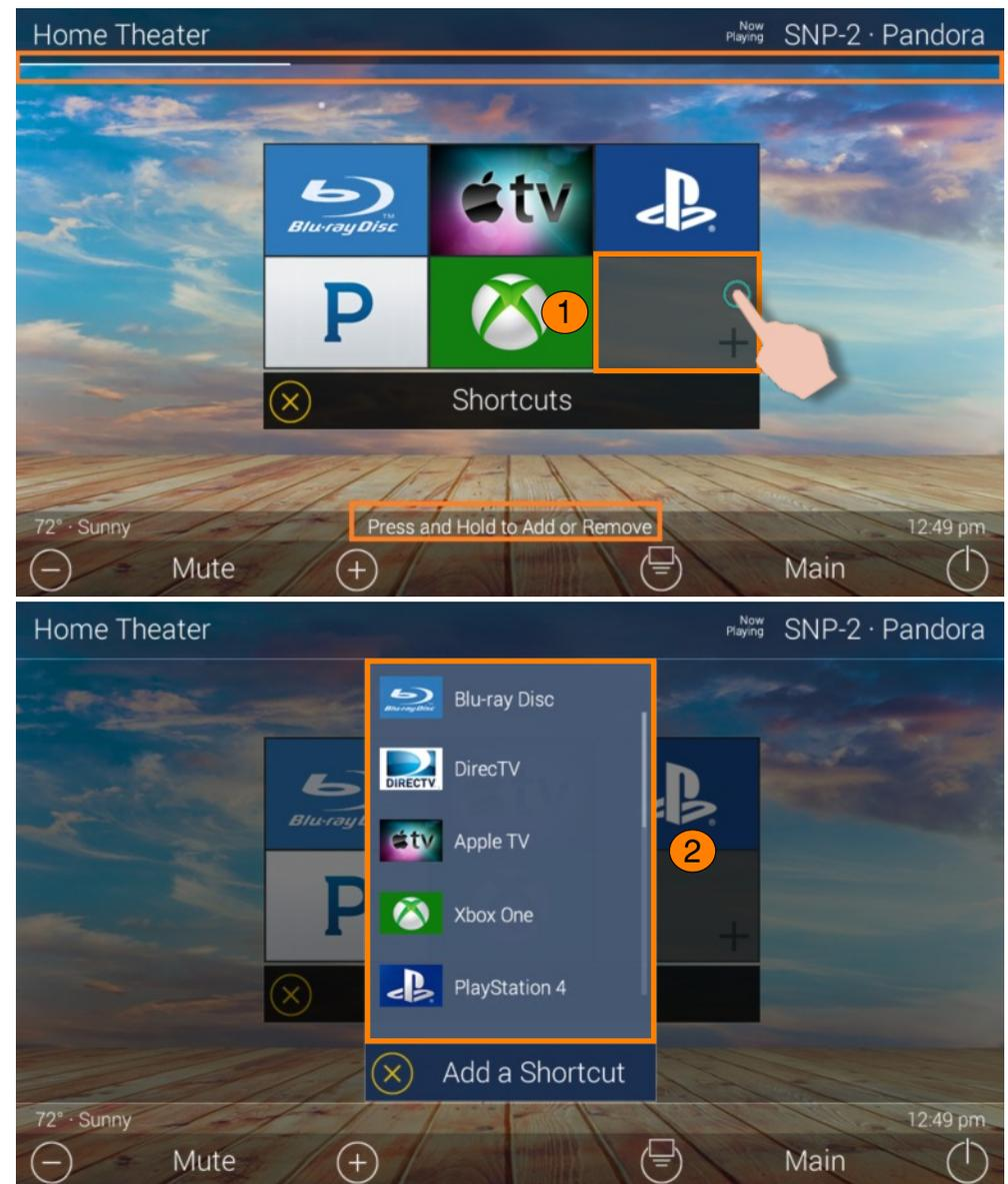
Just tap on a Shortcut button to launch that device/activity. Remember, this menu can only hold up to six (6) items and each item must already be a device/activity programmed into that current room.
