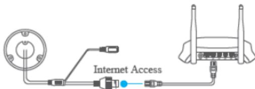
Figure 5-3 Connect a Router
