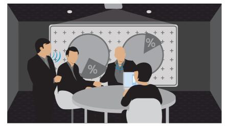
Suspending a microphone from the ceiling is another alternative. It has the advantage that the microphones can be installed virtually invisibly in the room. Ceiling installation requires precise prior planning, as the microphones are further away from the speaker and the speech intelligibility can be impaired by noise coming from the ventilator of a projector or from an air conditioning unit.
