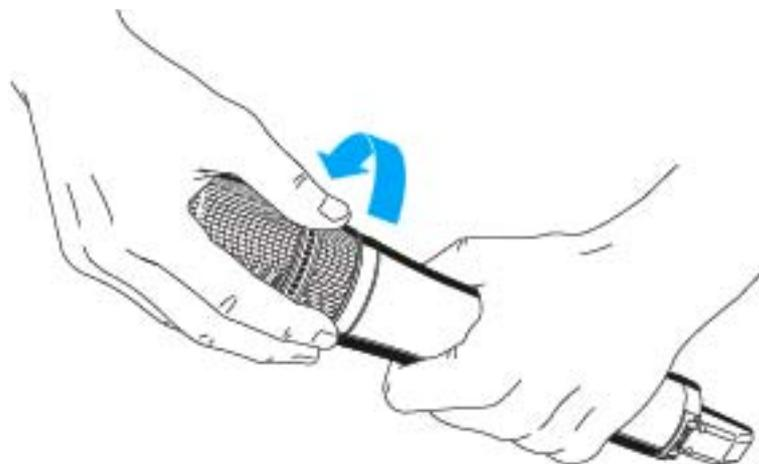
The microphone capsule can be unscrewed and replaced by one with a different pick-up pattern.
