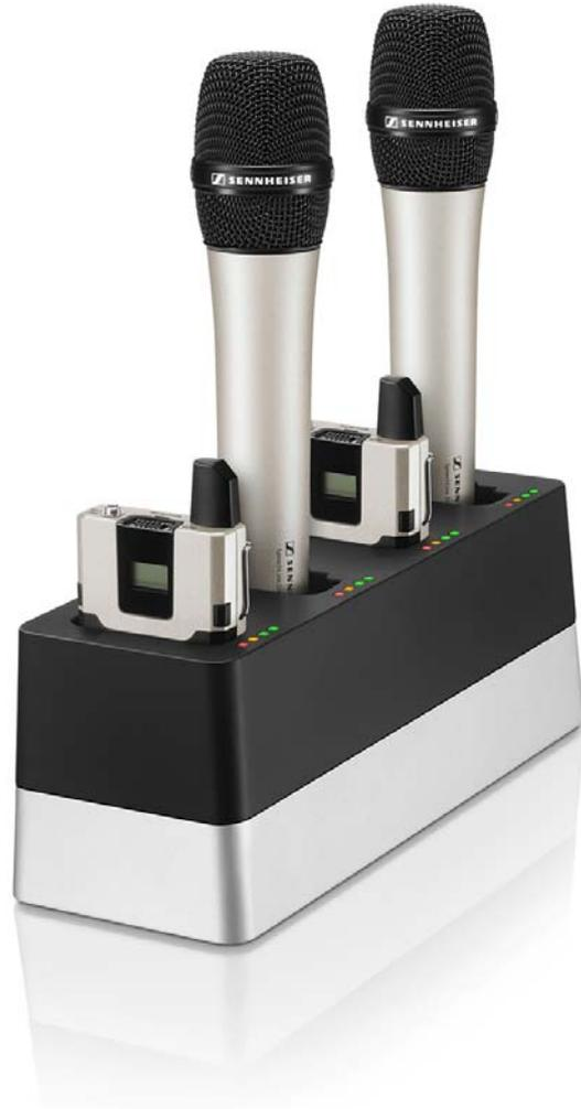
The CHG 4N is a network-compatible charger with four separate charging slots. These ports can be used for the SL Bodypack DW and the SL Handheld DW. The four LEDs on each charging slot indicate the current charging status. The versatile network interface is compatible with IPv4 and IPv6 for seamless integration. The Sennheiser Control Cockpit software can be used to monitor and remotely control the settings and status messages.
