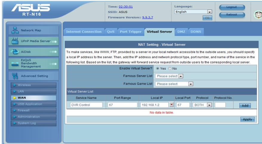
4. For Service Name, enter the name of the SnapAV product and the port function (example: Wirepath DVR Control Port). Enter the port number or range of numbers (example: 67-68) to be used in the Port Range field. For Local IP, select the Static IP address that was assigned to the SnapAV IP product during the initial SnapAV IP product setup. Protocol should be set according to the instructions for the port function, either TCP, UDP, or BOTH.
