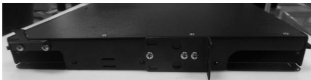
3. Install cable entry clamp on either left or right rear depending on feeder cable entry using supplied screws
