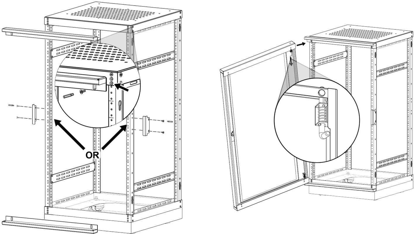
Note: The door may be installed for left- or right-hand swing. The hinge brackets are held on by 1 screw in each corner. The brackets are also slotted so that they can be adjusted for optimal door fit.
