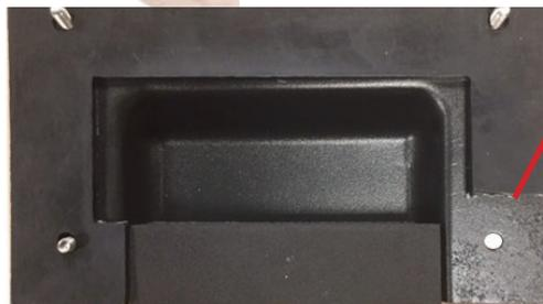
5. Trim gasket on Cable Cover by using razor knife or scissors) approximately 1" from the bottom as shown (Figure 2).
