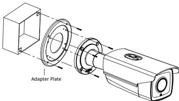
Figure 2-9 Installation with a Gang Box
