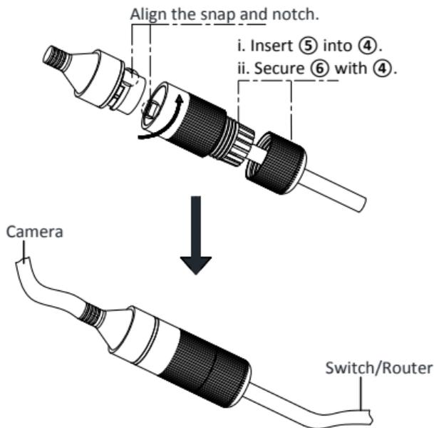
Figure 2-11 Water-proof Accessory Installation
