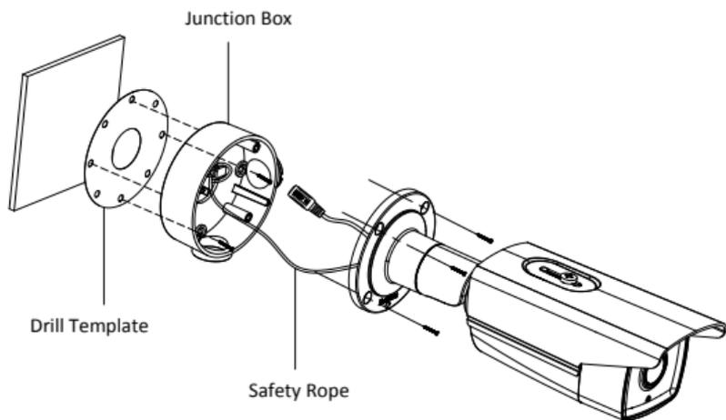
Figure 2-8 Installation with a Junction Box
