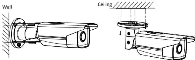
Figure 2-4 Install the Camera
