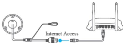
Figure 5-3 Connect a Router
