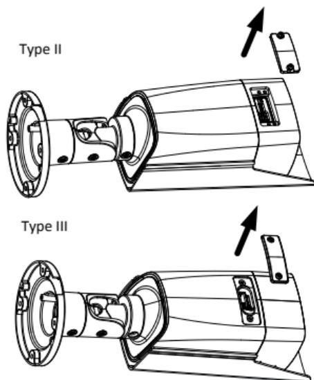
Figure 2-1 Expose Memory Card Slot
