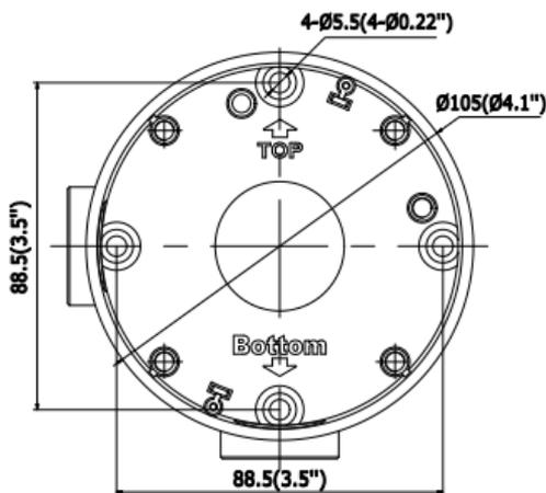
Figure 2-7 Dimension of Junction Box
