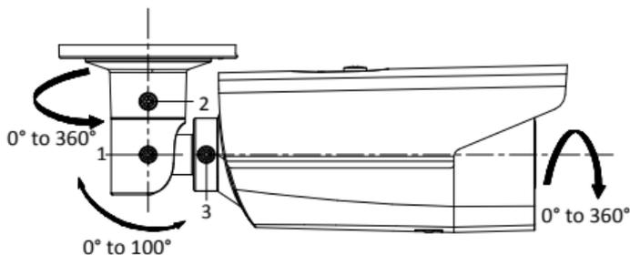
Figure 2-5 Adjust the View Angle
