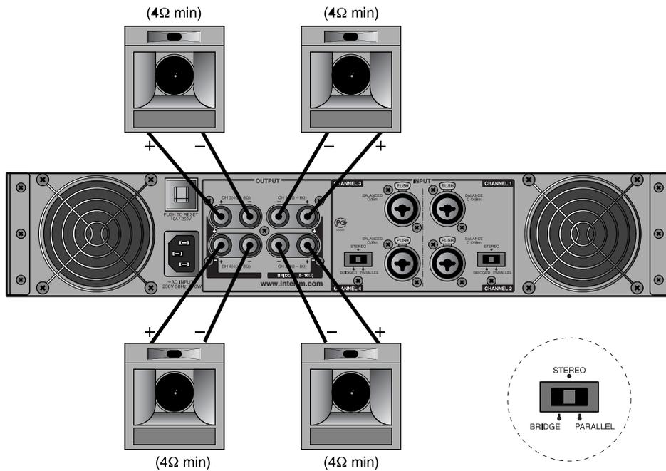
\* **CAUTION:** The parallel mode is the same connections with stereo mode, but you must set the switch to parallel mode and apply input to CH1 & CH3.
