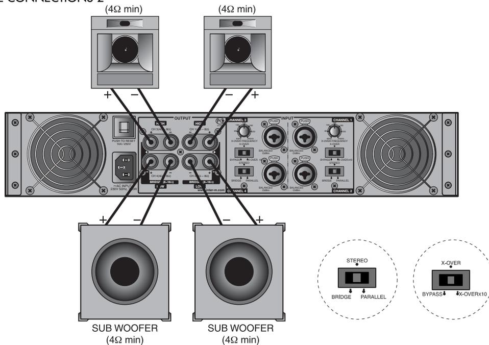
\* **CAUTION:** When you apply to X-OVER MODE, you must connect correctly for protecting speakers from being damaged. First, confirm output terminal on the rear panel of QX-4960, and then connect tweeter speakers to CH1 & CH3 output and woofer speakers to CH2 & CH4 output.
