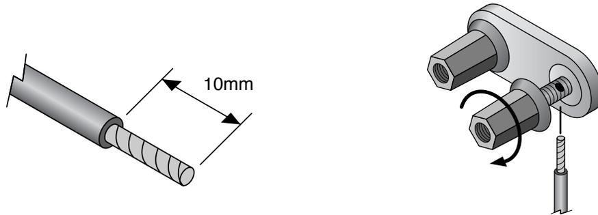
Make certain the wires do not protrude from the terminals and touch the amplifier's chassis, or an adjacent terminal.
