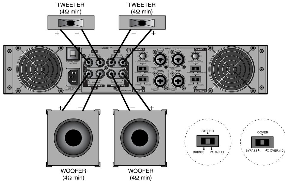
\* **CAUTION:** When you apply to X-OVER MODE, you must connect correctly for protecting speakers from being damaged. First, confirm output terminal on the rear panel of QX-4960, and then connect tweeter speakers to CH1 & CH3 output and woofer speakers to CH2 & CH4 output.
