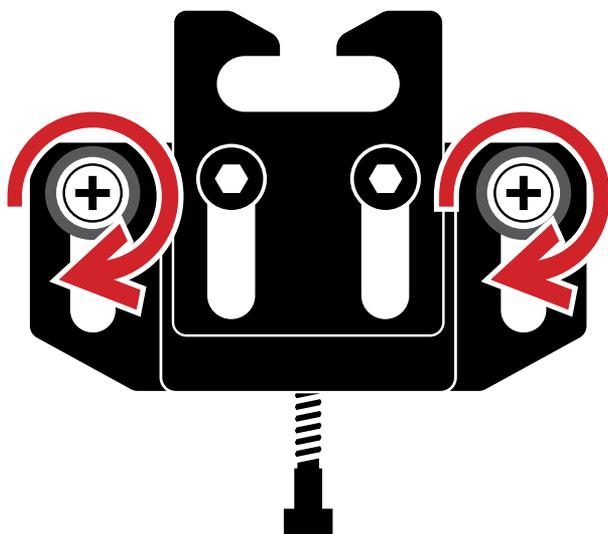
Remove **Templates** and attach **Brackets** to wall with **Wood Screws** or **Drywall Anchors**
