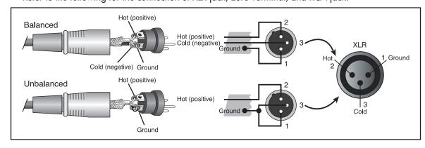
Turn PHANTOM switch OFF if using the unbalanced cable.
