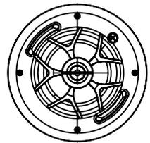
7. Fit the grille onto the speaker. **(See Figure I)**
