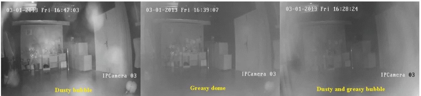
If the glass dome is dirty, the dirt can reflect infrared into the camera lens.
