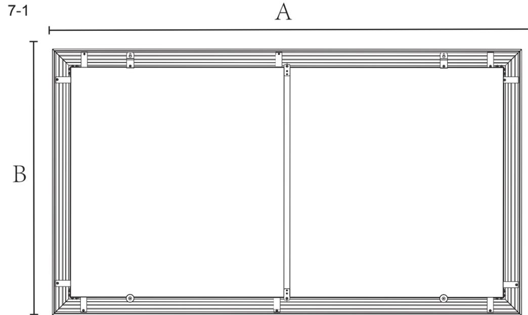
Drill 4 holes in the wall at the desired height. The two holes horizontal distance should be  $\frac{2}{3}A$ , the vertical distance should be  $B - 4\frac{1}{8}"$  (105mm).
