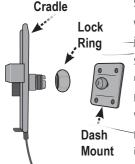
Slide the Lock Ring around the Dash Mount ball joint
