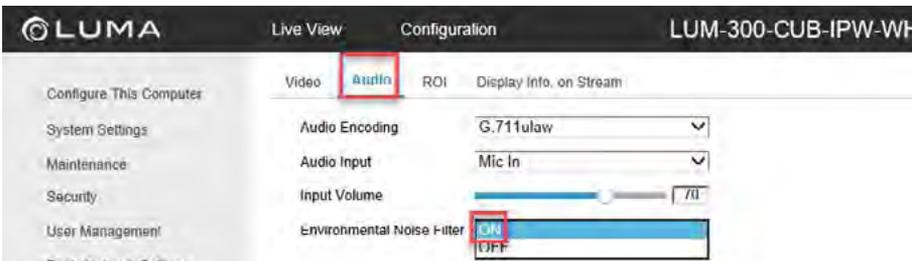
The screenshot shows the LUMA web interface Configuration page for camera LUM-300-CUB-IP, now on the 'Audio' tab. The 'Audio' tab is highlighted with a red box. The 'Environmental Noise Filter' dropdown menu is open, and 'ON' is selected, also highlighted with a red box. Other settings visible include Audio Encoding (G.711ulaw) and Audio Input (Mic In).
