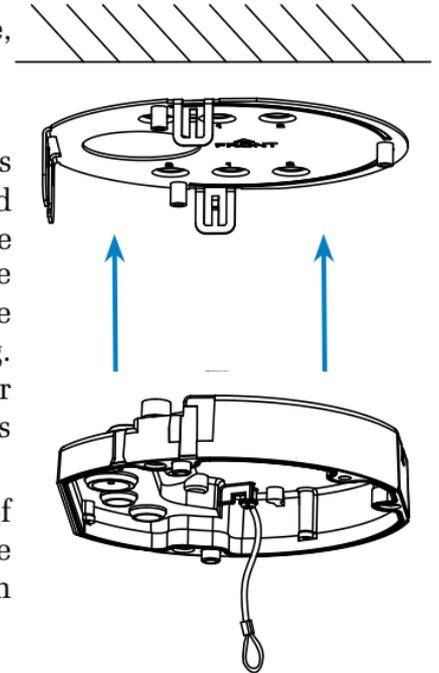
5. Connect all cabling to the camera. You can use the lanyard on the camera base to hang the camera on the hook inside the waterproof housing.
