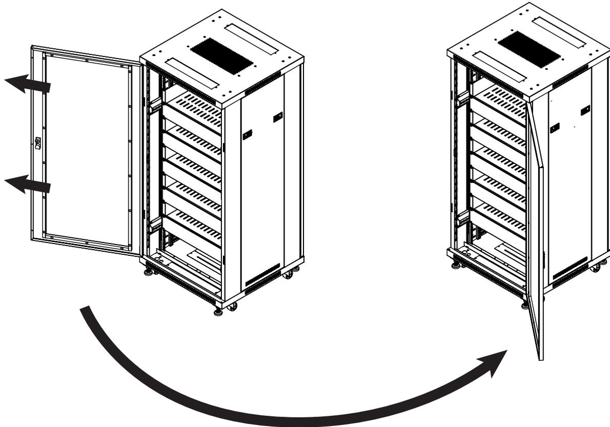
1. Open the door and pull the hinge pins free, then slide the door out of the rack.
