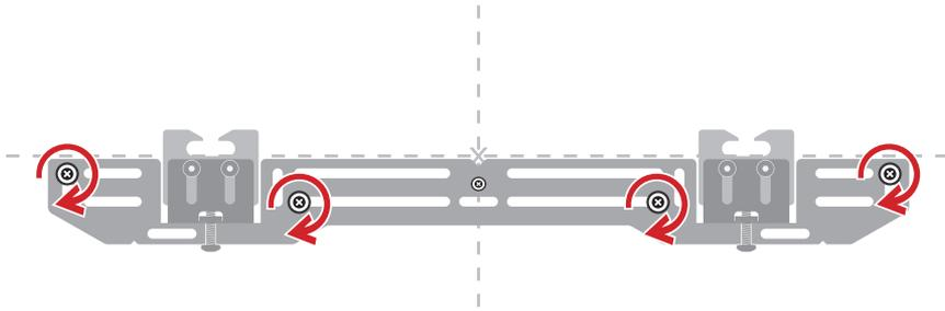
Secure **Bracket** to wall using **Bonded Washers** with **Wood Screws** or **Drywall Anchors**
