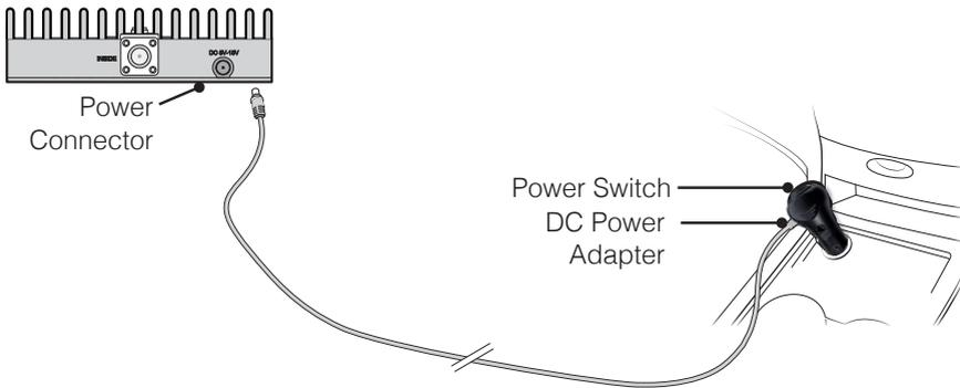
[1] WARNING: The booster is rated for 5-15V input voltage. DO NOT use the booster with a higher voltage power supply. This can damage the booster and/or cause personal injury.
