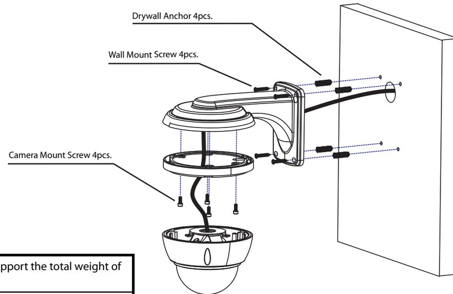
**!** Make sure to install in an area that can support the total weight of the camera and accessories.
