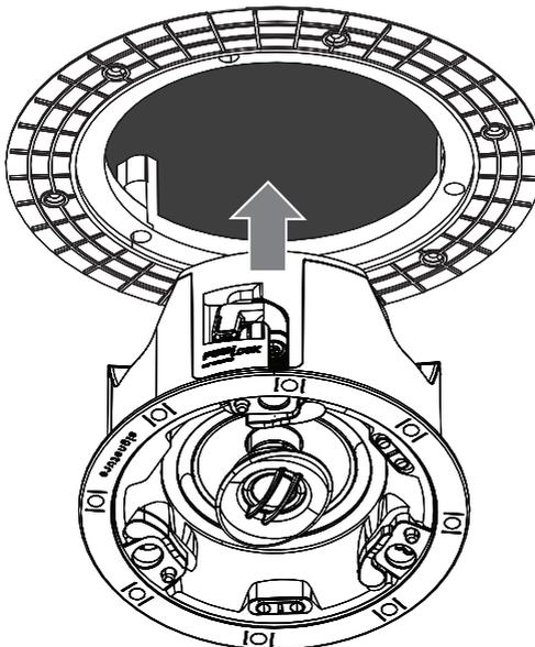
8. Remove the speaker and install the mud guard. Apply drywall mud over the bracket to seal and blend the bracket into the ceiling or wall.
