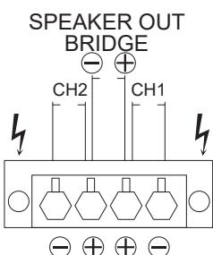
Use 14 or 16 gauge stranded two-conductor speaker wire. Connect the appropriate conductor to each screw terminal, observing correct polarity. Bridged markings are also shown to the left. Use burial rated wire as necessary for outdoor applications.
