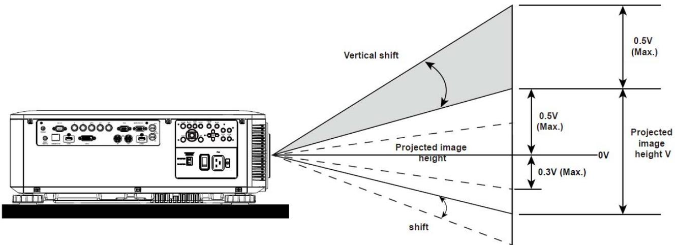
The projector is mounted on ceiling, the projected image can be moved down by 50% (0.5V) and up by 30% (0.3V).
