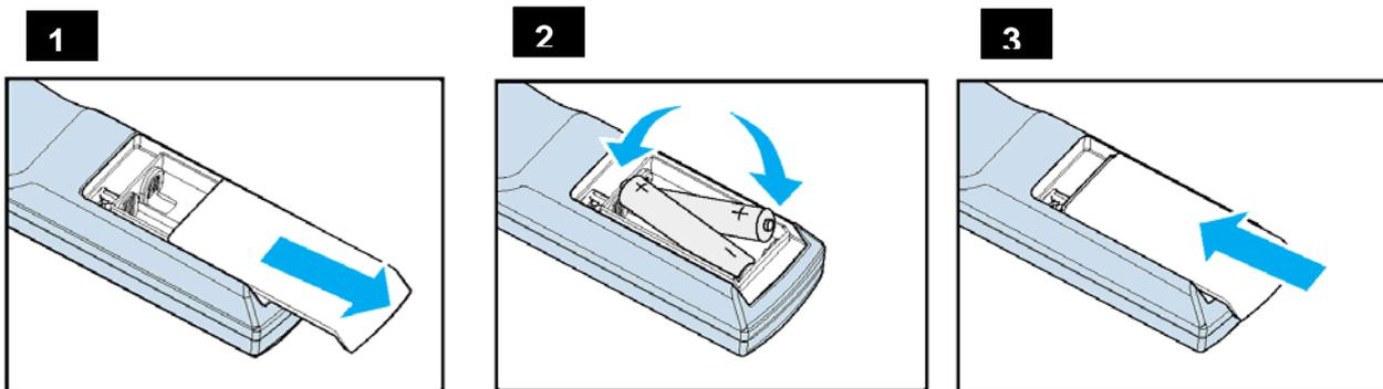
1. Remove the battery compartment cover by sliding the cover in the direction of the arrow.
