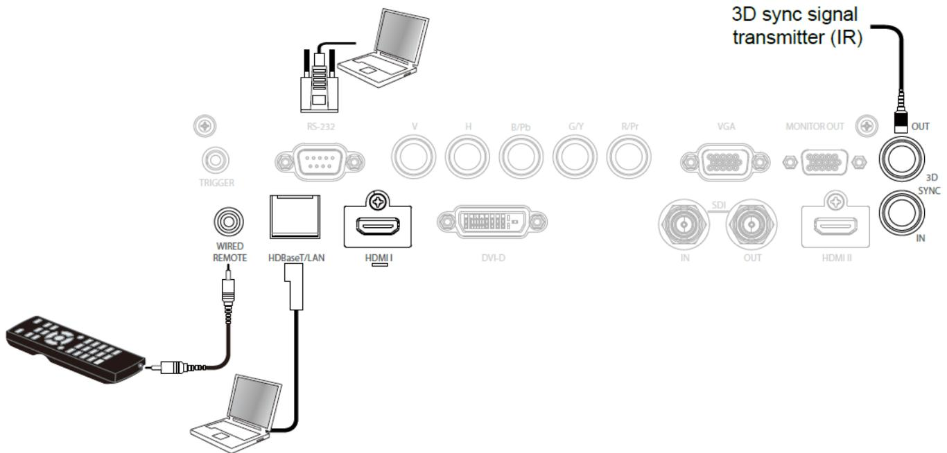
**HDBaseT/LAN (Network control):** The projector supports network control. LAN and Digital share the port. If only network control is used, you can connect the LAN on the projector to PC or through the local network. Refer to the remote control guidelines for
