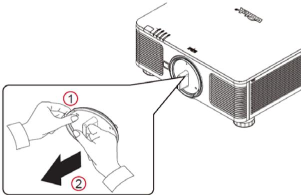
2. Align the "↑" symbol on the lens label with the "\*" symbol on the top of the body (align to the center of the lens hole) and pull in the lens.
