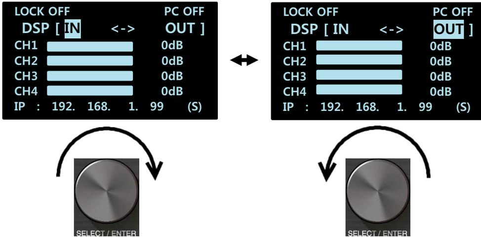
If you press down the SELECT/ENTER (ENCODER) dial after navigating to the item you want to adjust, you will be redirected to the sub-settings of the particular item. You can adjust the GAIN for each channel between -50.0dB and 00.0dB. You can change the integer and the decimal points separately. Also, the integer and decimal points that can be adjusted will be highlighted with a white background as shown in the above image.
