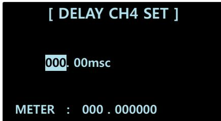
In DELAY settings, you can set the DELAY value for each channel. You can set values between 0.00 and 340.00msc in 48 Steps for each channel. Specifically, you can set the value you want down to the second decimal point. The initial value is set to 0.00msc. If you set the DELAY value, the approximate value of the corresponding distance is displayed at the bottom in METER units.
