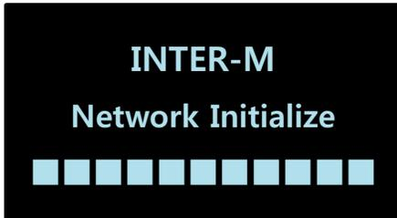
This initial screen appears when the power cable is connected to the set and the DSP begins to boot up. It indicates that the device is currently booting up. Boot-time is approximately 10 seconds.
