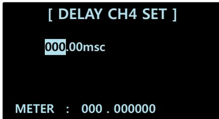
In DELAY settings, you can set the DELAY value for each channel. You can set values between 0.00 and 100.00msc in 48 Steps for each channel. Specifically, you can set the value you want down to the second decimal point.
