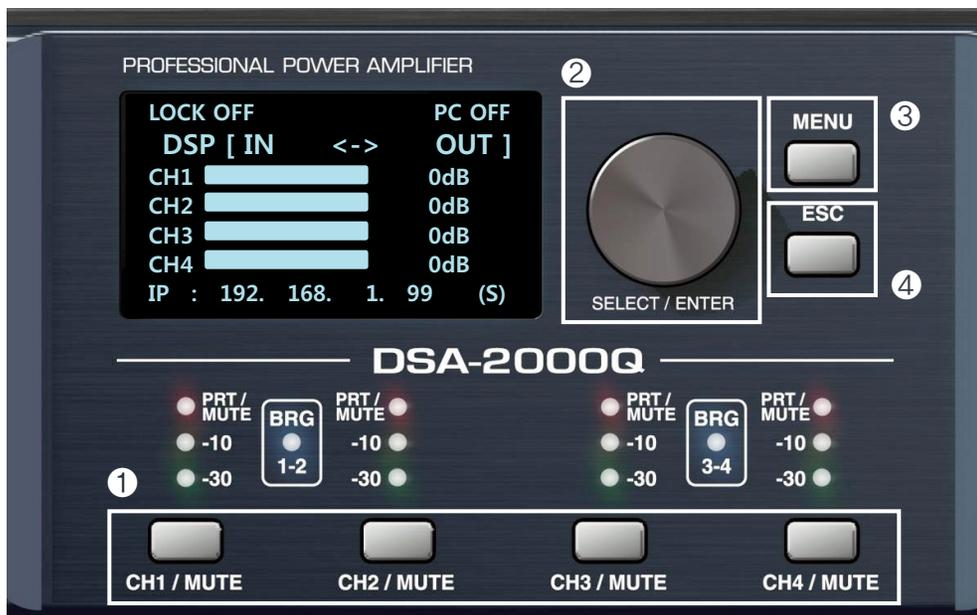
The above screen appears once the power is connected, booting is complete, and the power switch has been turned ON. It displays the volume and IP address for each channel, and you can check the connection status of your PC.
