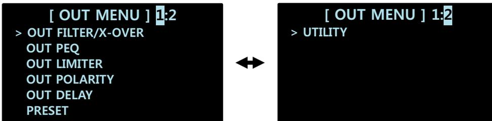
The OUT MENU features multiple items including OUT FILTER/X-OVER, OUT PEQ, OUT LIMITER, OUT POLARITY, OUT DELAY as well as PRESET and UTILITY. PRESET, UTILITY items are also available in the IN MENU.
