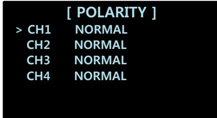
In POLARITY settings, you can set up each channel differently. You can configure each channel to NORMAL (normal phase) and INVERT (inverted phase), If you select INVERT, the phase will be inverted 180°. Initially, all channels are set to NORMAL.
