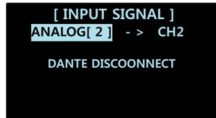
In SOURCE settings, you can distribute the audio signal received through the XLR INPUT/LINK terminal at the back of the device or through the network and the DANTE Digital Audio PORT to the output channel (speaker connection terminal) you want to use. Initial configuration: ANALOG[1]->CH1, ANALOG[2]->CH2, ANALOG[3]->CH3, ANALOG[4]->CH4. You can select from 8 SOURCES, including ANALOG [1]~[4], DANTE [RX0]~[RX3], etc.
