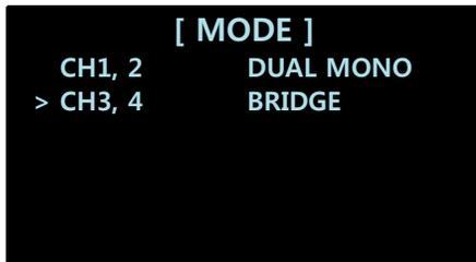
In MODE settings, you can select 5 different modes: DUAL MONO, STEREO, BI-AMP 1, BI-AMP 2, and BRIDGE. Initially, CH1, 2, 3, 4 are all set to DUAL MONO.
