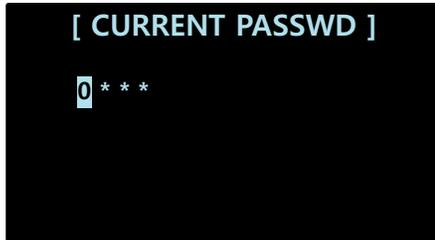
In PASSWD CHANGE, you can configure the password for the current device. You can select 4 numbers from 0 to 9. Turn the SELECT/ENTER (ENCODER) dial at the front of the device left/right to select the number you want. Once you have changed the password, press down the SELECT/ENTER (ENCODER) dial at the front to save your new password.
