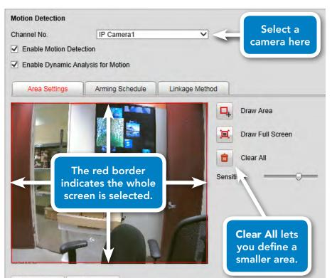
Select a camera in the dropdown at the top, and ensure motion detection is enabled with the checkbox.
