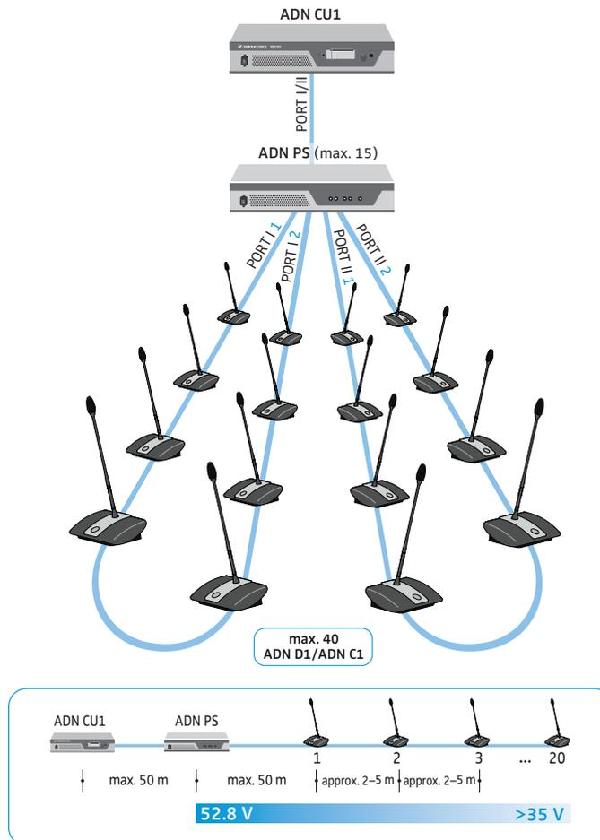
**i** When connecting the conference units to an ADN PS power supply, you can mix different cable topologies (simple cabling with cable strings or redundant ring topology) as long as you ensure correct cabling and comply with the specifications.
