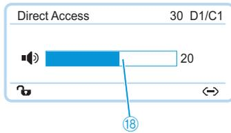
You can set the volume of the conference units' built-in loudspeakers via the jog dial on the central unit. The standard display displays the current volume setting 18.
