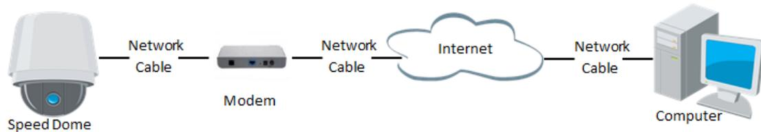
Figure 2-12 Accessing the Speed Dome with Dynamic IP
