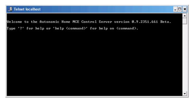
If you don't get a connection to the service, double check the Server Port setting in the configuration utility (MCS software), or check the server's IP configuration using the Mirage Media Server browser configuration pages.
