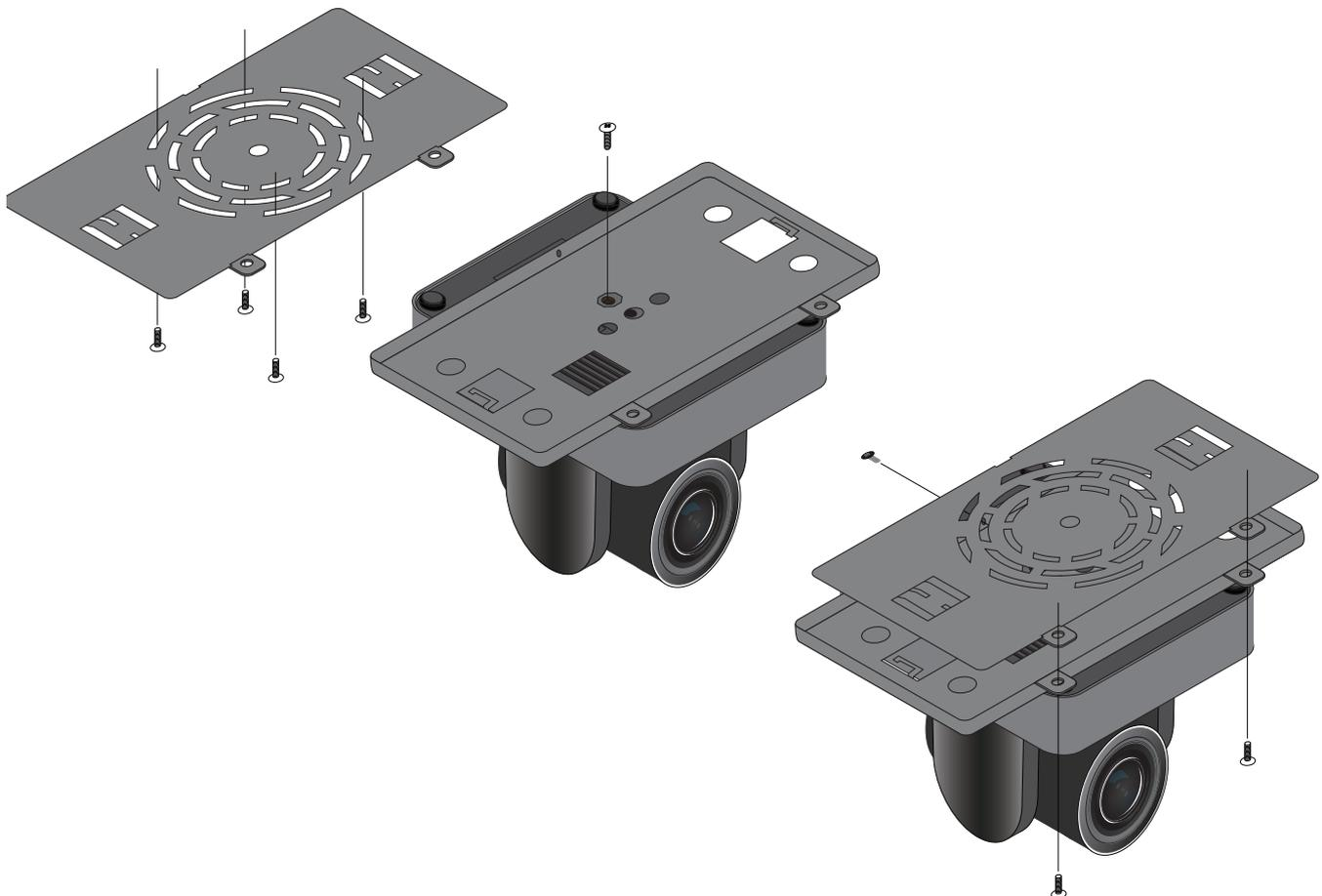
**i NOTE:** The camera picture will need to be inverted for video to be viewed correctly. Video can be inverted from the **Picture Settings** in the webGUI or using the **visca commands**.
