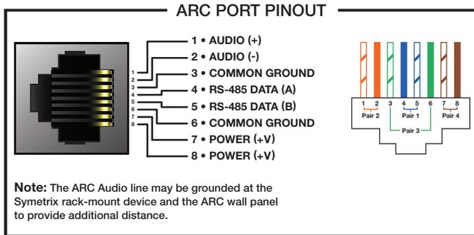
The Symetrix ARC-PSe provides serial control and power distribution over standard CAT5/6 cable for systems with more than 4 ARCs, or, when any number of ARCs are located long distances from a Integrator Series, Jupiter or Symetrix DSP unit.
