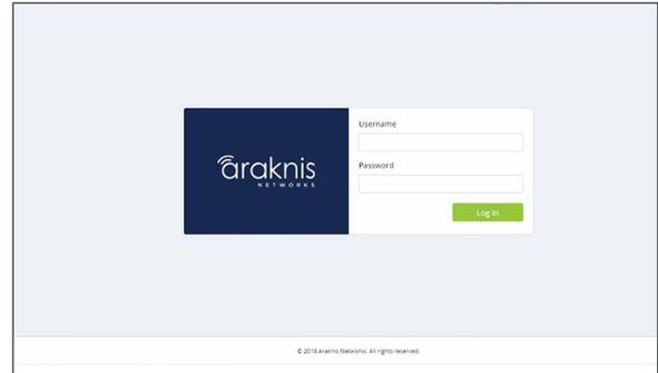
If you can't get to the login page, check to make sure your computer has been issued an IP address by the router. You can also claim the router in OvrC and use web connect.
