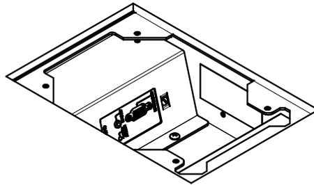
3. INSTALL COVER WITH SUPPLIED FLAT HEAD SCREWS.
