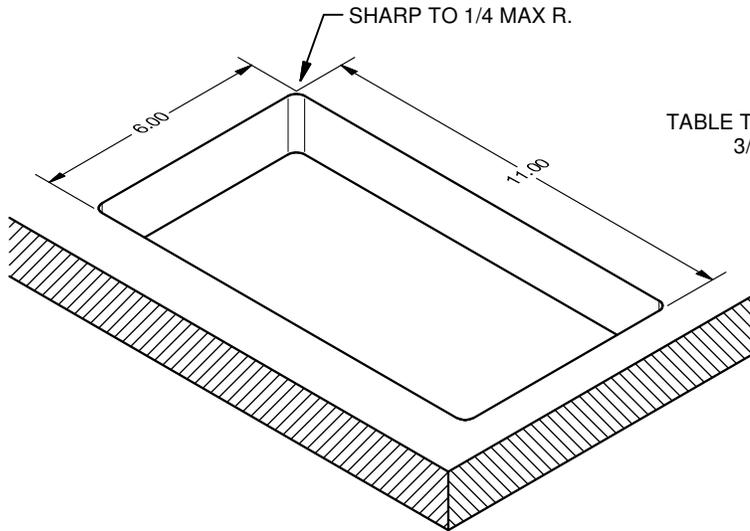
2. INSTALL DESIRED POWER UNITS/INTERNAL BRACKETS INTO RT6-RD4 ASSEMBLY. ADJUST HEIGHT OF UNITS/BRACKETS IN RT6-RD4 ASSEMBLY BEFORE INSTALLING IN THE TABLE. FOLLOW THE UNIT/BACKET INSTALLATION INSTRUCTIONS WHEN PROVIDED. IF RETRACTORS WILL BE INSTALLED, LEAVE THAT COMPARTMENT OPEN; RETRACTORS WILL BE ASSEMBLED LATER INTO A CASSETTE THEN INSTALLED FROM BOTTOM.
