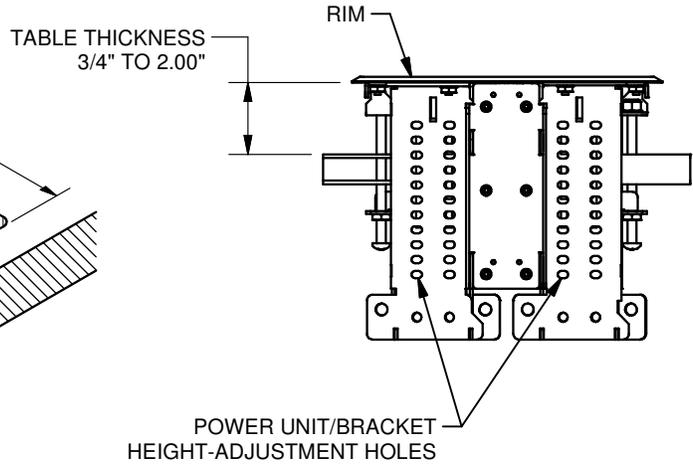
3. ROTATE LOCKING ARMS CLEAR OF TABLE AND INSERT RT6-RD4 ASSEMBLY INTO HOLE OF TABLE.
