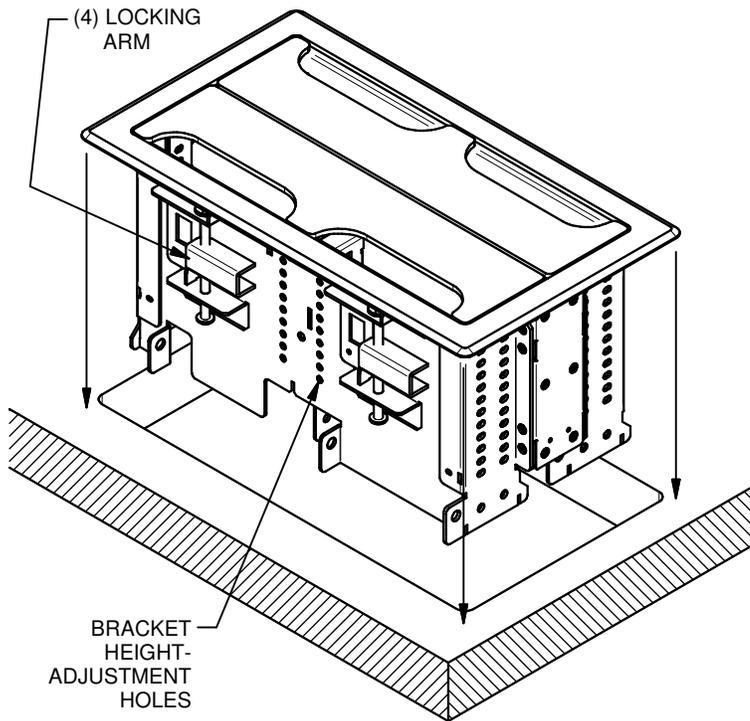
4. ROTATE LOCKING ARMS TO SECURE ASSEMBLY TO TABLE WITH ADJUSTMENT SCREW. LOCK ADJUSTMENT SCREW WITH INTEGRAL NUT WHERE NEEDED. MAKE ELECTRICAL CONNECTIONS AS REQUIRED.
