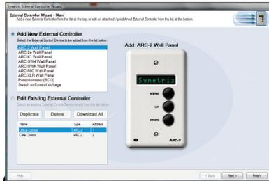
The **External Control Wizard** quickly configures ARC Wall Panels and the External Control inputs.
