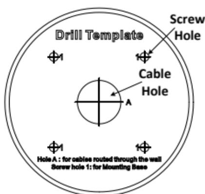
Figure 2-12 Drill Template of the Junction Box
