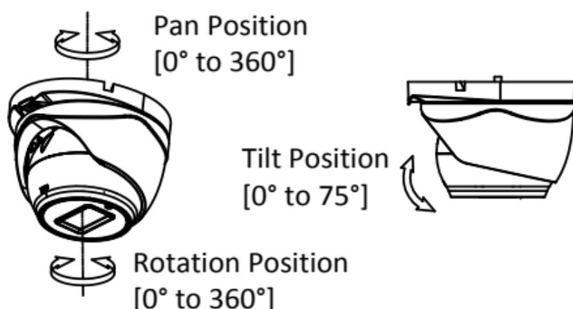
Figure 2-11 3-axis Adjustment
