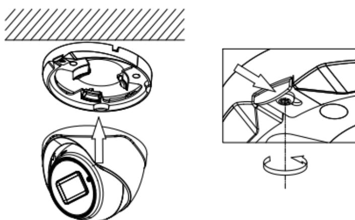
Figure 2-10 Install the Turret Camera
