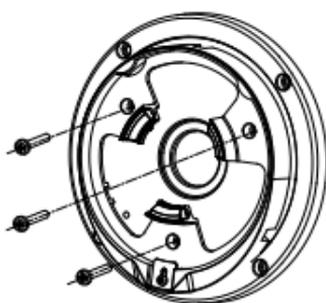
Figure 2-13 Secure Screws on Junction Box's Cover
