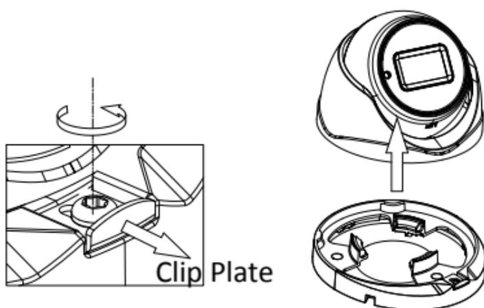
Figure 2-8 Remove the Clip Plate
