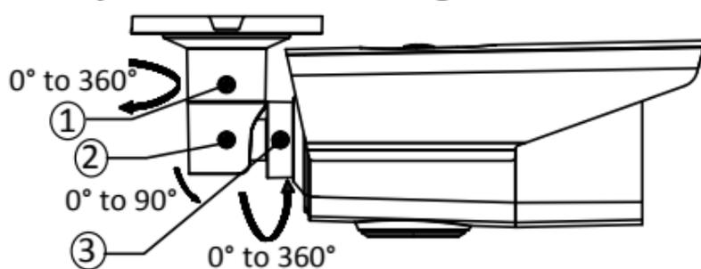
Figure 2-3 3-axis Adjustment
