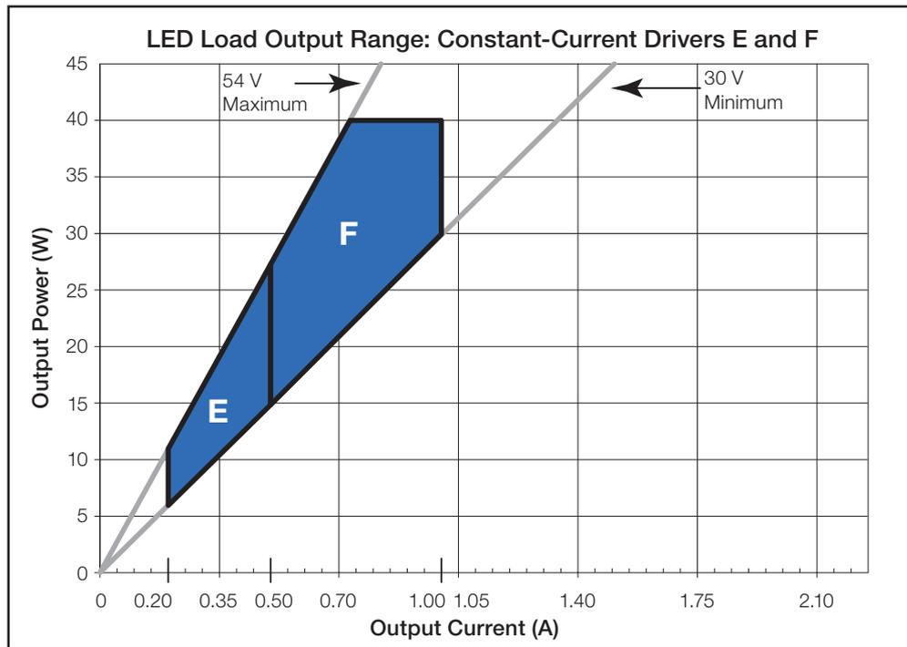
3A = Covers “LED Load Output Range” E and F (CCR dimming only)
