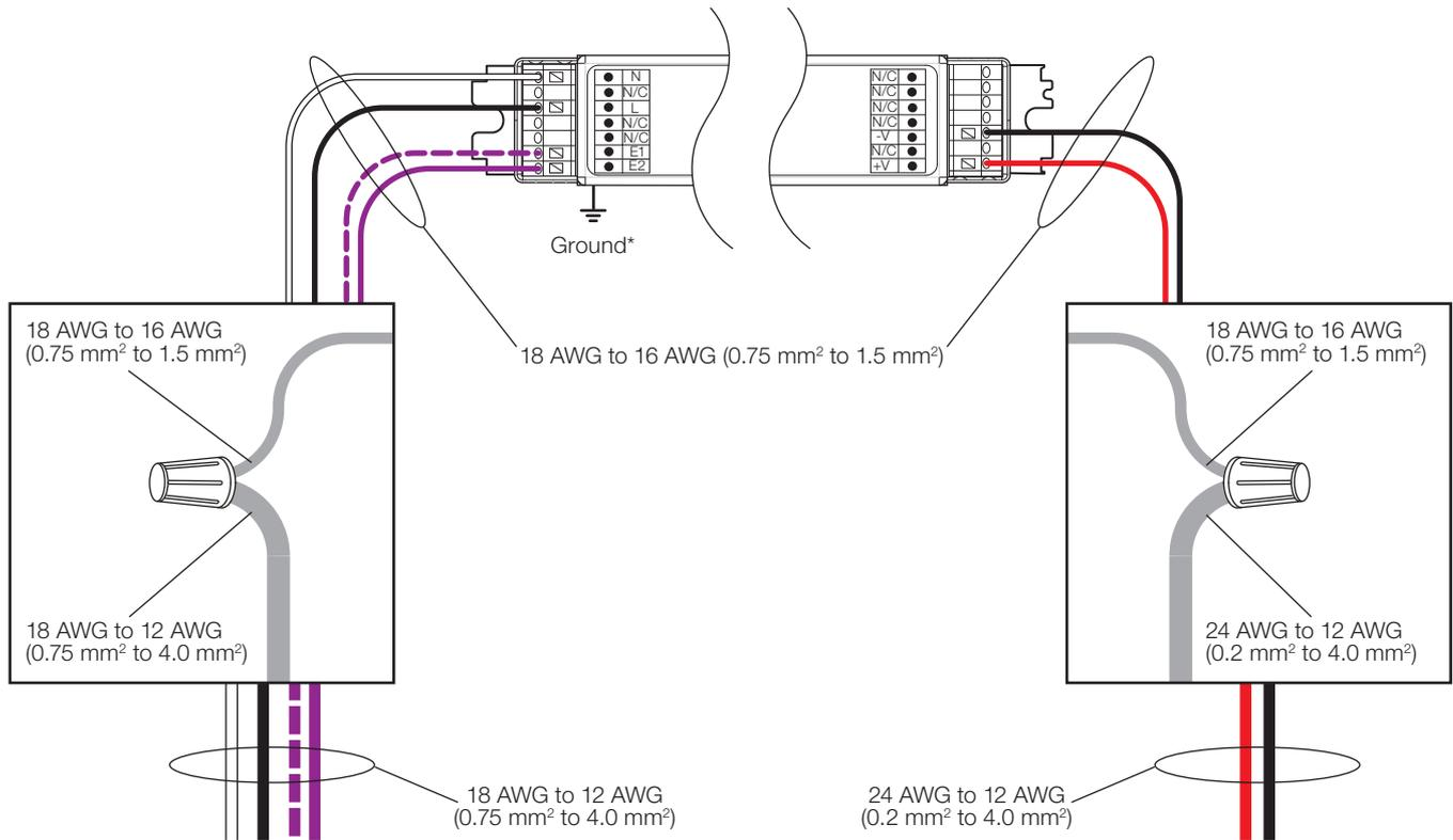
\* Fixture and driver case must be grounded in accordance with local and national electrical codes. Ground connection to driver case can be accomplished through ground terminal, and/or grounding the case. Ground connection to M case driver (shown) requires connection to stud in fixture.
