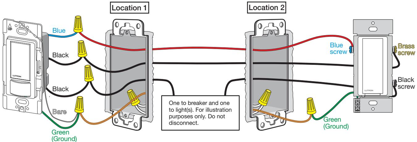
Note: Sensor switch must be grounded for the sensor to operate.
