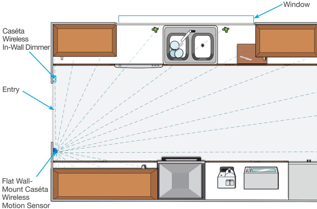
\* DO NOT place sensor within 4 ft (1.2 m) of moving air currents (e.g., HVAC vents), heat source (e.g., light bulbs or microwave/ standard ovens). Heat from an oven may cause sensor to see movement. Changing the activity setting to medium- or high-activity may be necessary. Refer to the back of the sensor or visit: [www.casetawireless.com/sensorfeatures](http://www.casetawireless.com/sensorfeatures)
