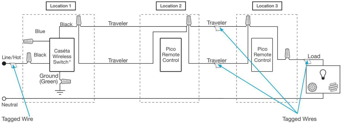
\* It is recommended to install in-wall switch in either Location 1 or 3.
