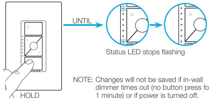
NOTE: Changes will not be saved if in-wall dimmer times out (no button press for 1 minute) or if power is turned off.
