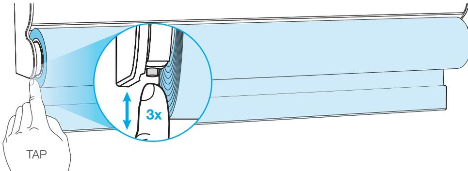
**NOTE:** The "Shade" button LED will flash GREEN-then-RED three times, signaling the successful completion of the procedure.
