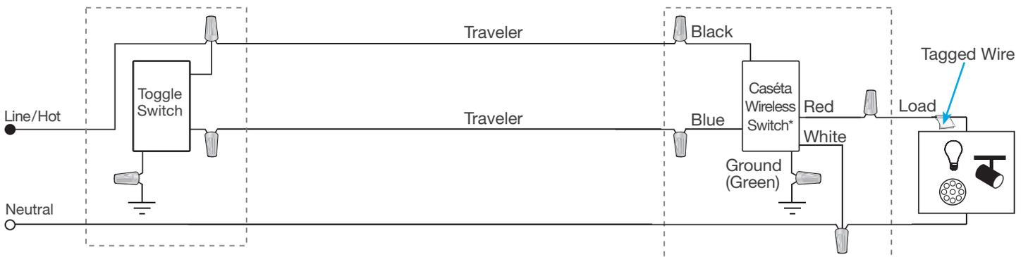
\* Switch may be installed in either location.
