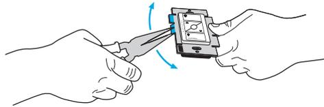
**Do not** remove outside side sections on dimmers at the end of gang.
