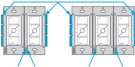
Each control has inside side sections removed.
