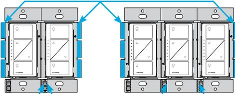
Each in-wall dimmer has inside side sections removed.
