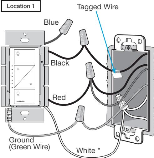
\* If available, connect the neutral wire from the wallbox to the white wire on the in-wall dimmer. If neutral is not available, cap the white wire with a wire connector. *Neutral required for: MLV loads, LED drivers, PHPM-PA, PHPM-3F, GRX-TVI.*
