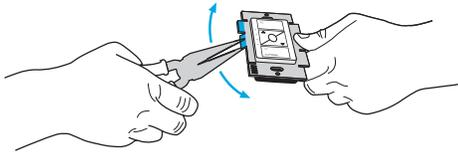
**Do not** remove outside side sections on fan controls at the end of gang.
