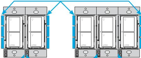
Each in-wall switch has inside side sections removed.
