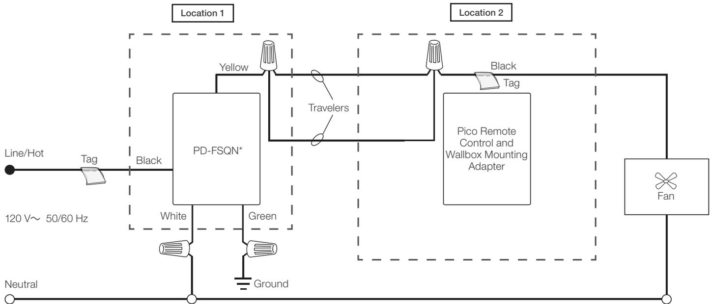
\* Control can be installed in either location.
