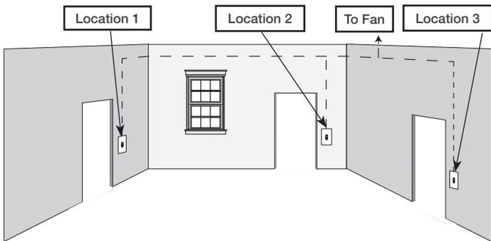
Three or more switches control the fan (multi-location installation)
