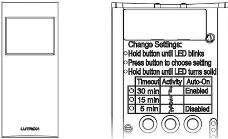
The motion sensor has several advanced set-up features. For the majority of installations, the default settings will provide the best performance and you will not need to utilize the advanced set-up. The motion sensor has three adjustable advanced set-up modes: Timeout, Activity, and Auto-On.
