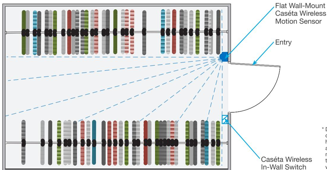
\* DO NOT place sensor within 4 ft (1.2 m) of moving air currents (ie: HVAC vents), heat source (ie: light bulbs). Changing the activity setting to medium or high activity may be necessary. Refer to the back of the sensor or visit: [www.casetawireless.com/sensorfeatures](http://www.casetawireless.com/sensorfeatures)
