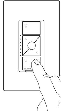
a. Tap "Off" button one time on in-wall dimmer control. Light will turn off.
