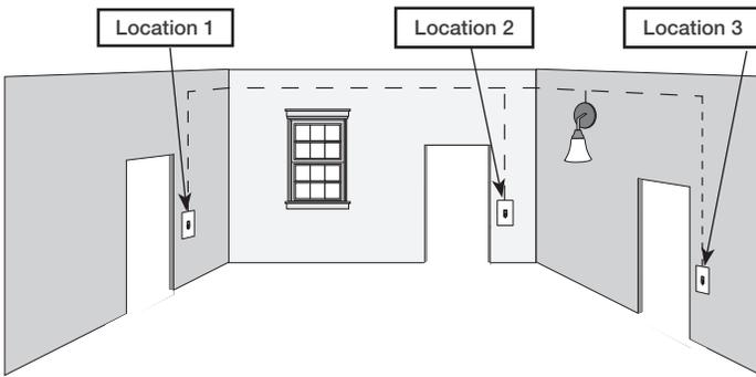
Three or more switches control the lights (multi-location installation)
