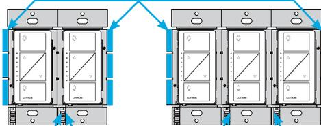
Each in-wall dimmer has inside side sections removed.
