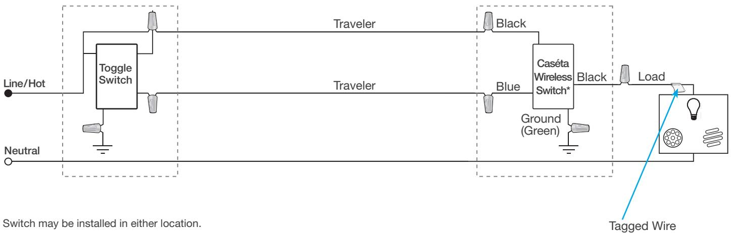
\* Switch may be installed in either location.
