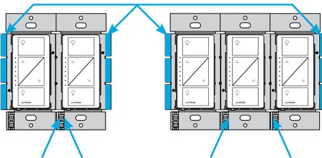
Each in-wall dimmer has inside side sections removed.
