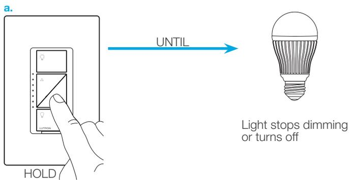
Light stops dimming or turns off
