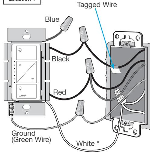
\* If available, connect the neutral wire from the wallbox to the white wire on the in-wall dimmer. If neutral is not available, cap the white wire with a wire connector. *Neutral required for: MLV loads, LED drivers, PHPM-PA, PHPM-3F, GRX-TVI.*
