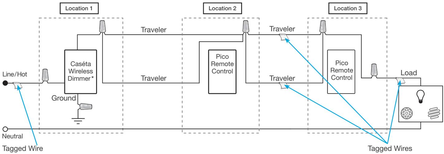
\* It is recommended to install in-wall dimmer in either Location 1 or 3.
