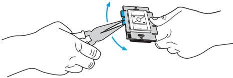
**Do not** remove outside side sections on the controls at the end of gang.
