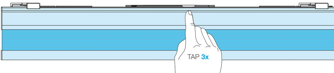
**NOTE:** The "Shade" button LED will flash GREEN-then-RED three times, signaling the successful completion of the procedure.
