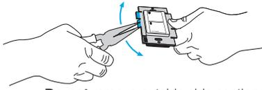
**Do not** remove outside side sections on switches at the end of gang.
